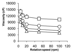
**Figure 2:** Rheograms of FDP ( $\square$ ), RDP( $\circ$ ) and RDP aged at 4°C ( $\diamond$ ) and 25°C ( $\Delta$ ) for 4 months.
