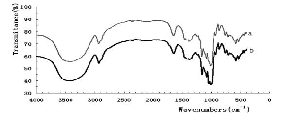
**Fig 1:** FTIR spectrum of sweet potato starch phosphodiester. *Key:* a = sweet potato starch; b = sweet potato starch phosphodiester
