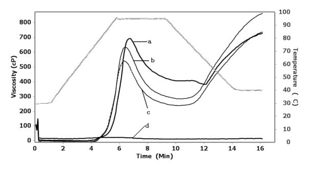
**Fig 3:** RVA curves of the samples. *Key:* a = sweet potato starch; b = sweet potato starch phosphodiester (RS23%); c = sweet potato starch phosphodiester (RS58%); d = sweet potato retrograded starch (RS100%)
