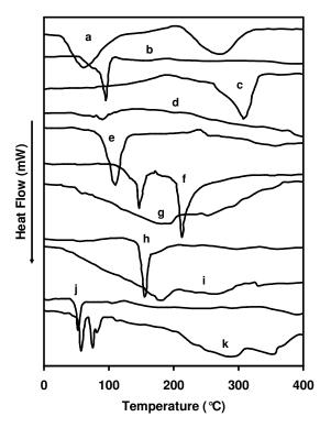
**Figure 2:** DSC Thermograms: (a) Sennosides; (b) sorbitol; (c) 1:1 sorbitol-sennoside mixture; (d) sodium carbonate; (e) 1:1 sodium carbonate-sennoside mixture; (f) Tablettose (lactose); (g) 1:1 lactose-sennoside mixture; (h) glucose; (i) 1:1 glucose-sennoside mixture; (j) stearic acid; (k) 1:1 stearic acid-sennoside mixture. The arrow indicates the direction of endothermic processes
