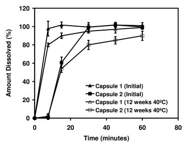
**Figure 4:** Initial dissolution profiles for the sennoside capsule formulations compared to the dissolution profiles after being stored for 12 weeks at  $40 \,^{\circ}\text{C} + 75 \,^{\circ}\text{C}$  RH
