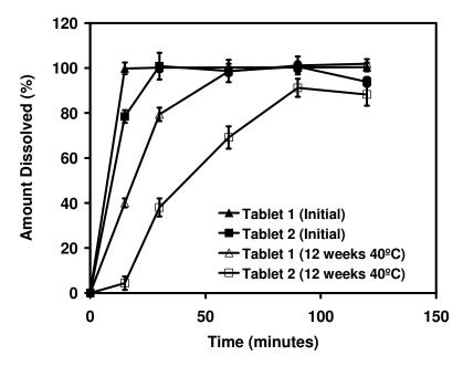
**Figure 5:** Initial dissolution profiles for the sennoside tablet formulations (Tablet 1 – direct compression; Tablet 2 – wet granulation) compared to the dissolution profiles after being stored for 12 weeks at 40  $^{\circ}$ C + 75  $^{\circ}$ RH
