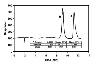
**Figure 1:** HPLC Chromatograms of Sennosides A and B. Parameters for linearity are shown on the figure. Retention time: Sennoside B = 9.4 min, Sennoside A = 10.9 min; Number of theoretical plates (N): Sennoside B = 7527 plates/column, Sennoside A = 6298 plates/column (Tangent method); USP tailing factor (T): Sennoside B = 0.95, Sennoside A = 1.04; Capacity factor (k'): Sennoside B = 1.68, Sennoside A = 2.09; Resolution between peaks: 2.98. 15.16
