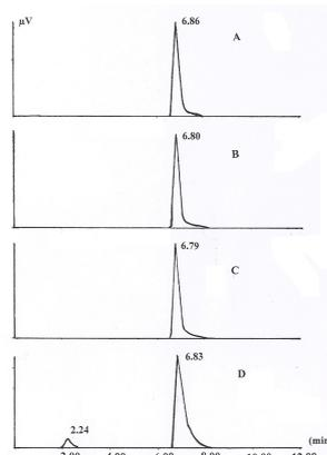
**Figure 1:** Chromatographic illustration of degradation products of MLX; (A) MLX; (B) Oxidative condition; (C) Basic condition; (D) Acidic condition
