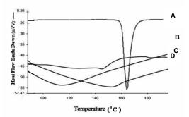
**Fig 4:** DSC thermograms of pure indomethacin (A) and chitosan films (B = F6, C = F11, and D = F1) (Code key as in Table 1)
