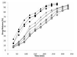
**Fig 2:** Release of indomethacin from chitosan films in pH 3.5 medium:  $\blacksquare = F1$ ;  $\square = F3$ ;  $\blacksquare = F5$ ;  $\blacktriangle = F6$ ,  $\triangle F8$ ,  $\blacktriangle F10$ ,  $\bullet F11$ ,  $\circ F13$ ,  $\bullet F15$  (See Table 1 code key)
