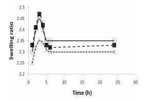
Fig 1: Swelling ratio of chitosan films ( $\circ$  = LMW, = MMW,  $\Delta$  = HMW) in pH 3.5 medium
