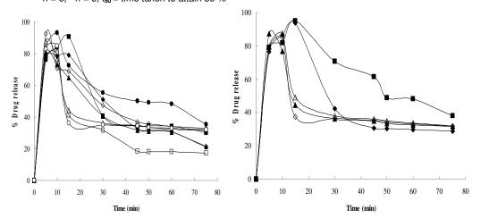
**Figure 1:** Dissolution profiles of artesunate tablet brands. (a):  $\blacklozenge = A$ ;  $\blacksquare = B$ ;  $\blacktriangle = C$ ;  $\diamondsuit = D$ ;  $\Box = E$ ;  $\blacklozenge = F$ ;  $\triangle = G$ ;  $\bigcirc = H$ ; and (b):  $\triangle = I$ ;  $\blacklozenge = B1$ ;  $\blacksquare = F1$ ;  $\blacktriangle = G1$ ;  $\diamondsuit = H1$
