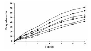
**Fig 3**: Effect of polymer type and ratio on the release of clotrimazole from bioadhesive vaginal tablets. *Key:* F1 ( $\diamond$ ), F2 (•), F3 ( $\Delta$ ), F4 (**■**), F5 (\*) and F6 ( $\blacktriangle$ )
