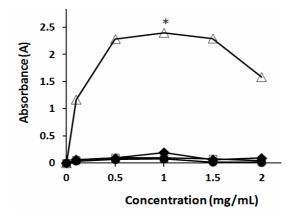
**Figure 5:** Reducing power (n = 3) of CS salts: CS-acetate ( $\blacklozenge$ ), CS-HOBt ( $\Box$ ), CS-TPP ( $\Delta$ ) and CS-EDTA ( $\bullet$ ); \* indicates significance difference at *p* < 0.05
