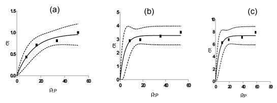
**Figure 2:** Plot of radial crushing strength against the product of pressure of compression pressure and relative density of *Saraca indica* bark for (a) powder (b) direct compression formulation, and (c) granules
