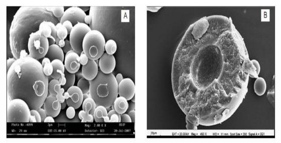
Figure 1: Scanning electron micrograph (SEM) of microballoons: (A) outer surface; (B) inner surface of a cross-section
