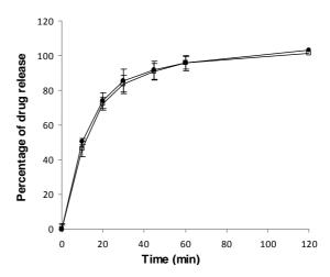
**Figure 4:** Clotrimazole dissolution profiles obtained by flow-through cell method in acetate buffer pH 5.2 containing 1 % SDS at a constant flow rate of 16 ml/min. The tablets were positioned uniformly in a clip holder (F1,  $\bullet$ ) or situated directly on the glass beads (F2,  $\blacksquare$ ). Each value represents mean  $\pm$  SD (n = 6).
