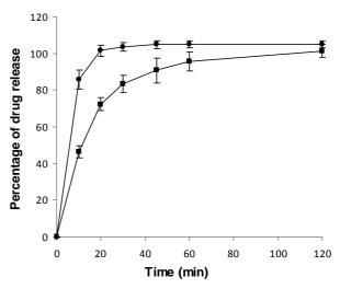
Figure 3: Clotrimazole dissolution profiles obtained by flow-through cell at constant flow rate of 16 ml/min.in 0.1M HCl ( $\bullet$ ) and acetate buffer pH 5.2 with 1 % SDS ( $\blacksquare$ ). Each value represents mean  $\pm$  SD (n = 6)
