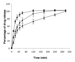
Figure 2: Clotrimazole dissolution profiles obtained by flow-through cell method in acetate buffer (pH 5.2) containing 1 % SDS at flow rate of 4 ml/min ( $\blacktriangle$ ); 8 ml/min ( $\bullet$ ); and 16 ml/min ( $\blacksquare$ ). Each value represents mean  $\pm$  SD (n = 6)
