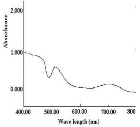
**Figure 1:** Spectrum of losartan–copper complex showing absorption maximum at 530 nm
