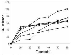
**Figure 5:** Dissolution of ketoprofen crystals. *Key:* Original ketoprofen =  $\Diamond$ , RS =  $\blacksquare$ , SC =  $\triangle$ , SA =  $\times$ , SD = -, and FD =  $\circ$
