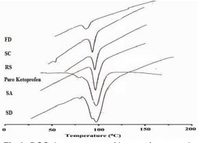
Fig 2: DSC thermograms of ketoprofen crystals
