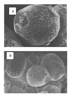
**Fig. 1:** SEM photographs of floating microspheres of (a) Cellulose Acetate (b) Eudragit RS100
