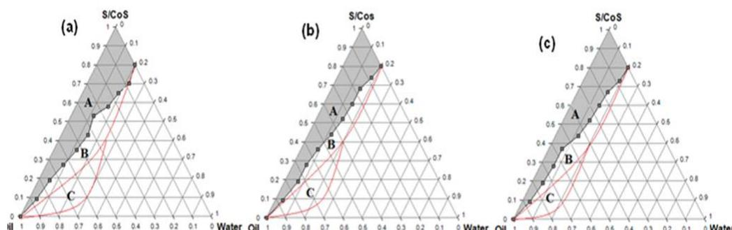
Figure 2: Pseudoternary phase diagrams of Capryol PGMC, Transcutol and PEG 400 with 100 mg of 5FU. a)  $S_{mix}$  1:1; b)  $S_{mix}$  2:1 c)  $S_{mix}$  3:1
