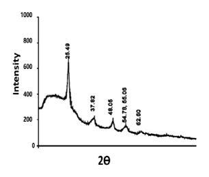
Figure 1: X-ray diffraction (XRD) peaks of greensynthesized titanium oxide nanoparticles
