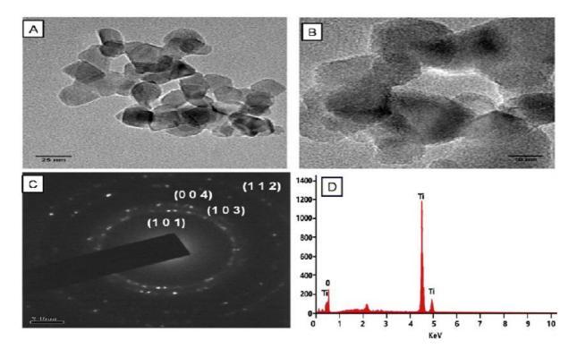
**Figure 2:** (A, B) Transmission electron microscopy (TEM) images of  $TiO_2$  NPs, (C) selected-area electron diffraction (SAED) pattern of the NPs, and (D) energy dispersive X-ray spectroscopy (EDS) profile showing the elements contained in the NPs
