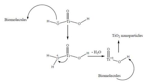
Figure 6: Plausible mechanism for the formation of TiO<sub>2</sub> NPs
