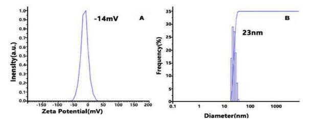
Figure 3: (A) Zeta potential value of TiO<sub>2</sub> NPs and (B) average size of the prepared NPs.
