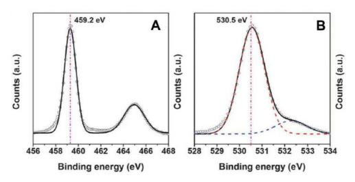
**Figure 4:** High-resolution x-ray photoelectron spectroscopy (XPS) spectra of (A) the titanium 2p peak and (B) the oxygen 1s peak of TiO<sub>2</sub> NPs
