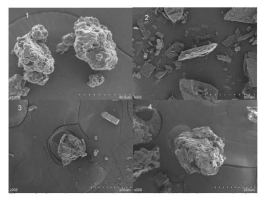
**Figure 3:** Scanning electron micrographs of lecithin(1), formononetin (2), their physical mixture (3) and complex (4)
