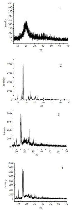
**Figure 5:** X-ray diffraction patterns of lecithin (1), formononetin (2), their physical mixture (3) and complex(4)
