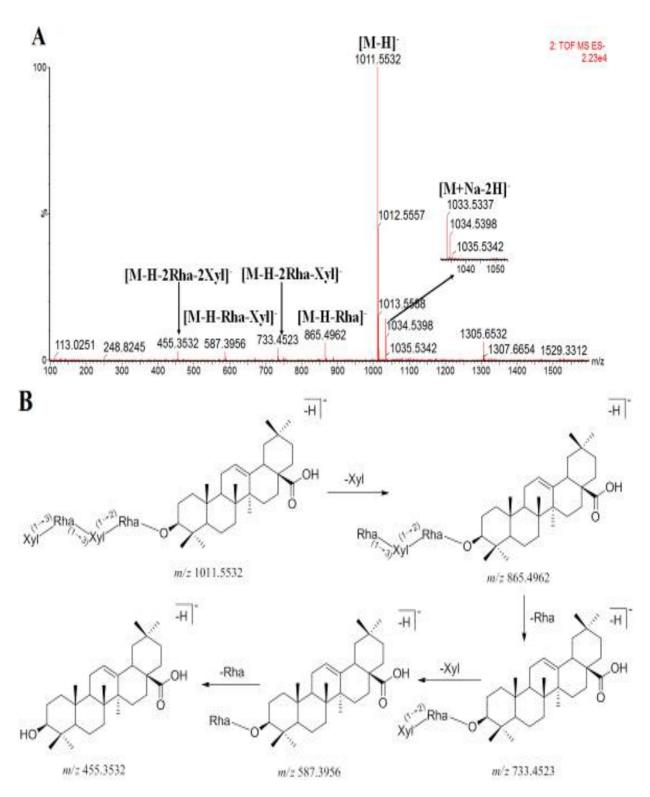
Figure 5: MS diagram (ESI-) and ions fragmentation pathways of triploside G (35)
