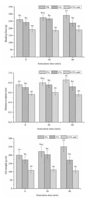
**Figure 2:** Distance to rupture, breaking force, and gel strength of the fish meat gels. Different letters (a, b and c) reflect significant differences (p < 0.05) among samples with different salt contents at the same sonication time. The letters x and y indicate significant differences (p < 0.05) between the two sonication periods at the same salt level
