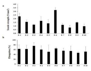
Figure 3: Tensile strength (a) and elongation (b) of patches
