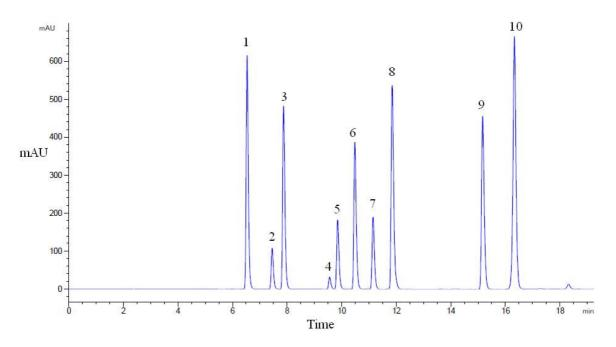
**Fig 2:** Resolution of chromatograms of synthetic dyes. 1 – Tartrazine; 2 - Quinoline yellow 1; 3 - Indigo carmine; 4 - Quinoline yellow 2; 5 - Ponceau 4R; 6 - Sunset yellow; 7 - Quinoline yellow 3; 8 - Allura red AC; 9 – Carmozine; 10 - Brilliant blue
