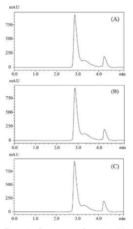
**Figure 2:** Chromatogram of standard (A), F7 formulation (B), and JointFlex<sup>®</sup> topical cream (C)
