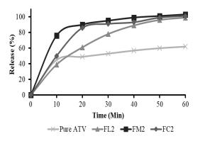
**Figure 2:** Cumulative release of solid dispersions prepared with fusion method at drug: carrier ratio of 1:2
