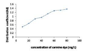
Figure 6: Effect of E120 dye concentration adsorption onto activated carbon
