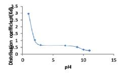
Figure 3: Effect of pH on E120 dye adsorption onto activated carbon
