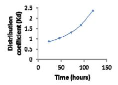
Figure 2: Effect of agitation time on E120 dye adsorption onto activated carbon
