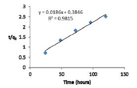
**Figure 10:** Pseudo second- order kinetics for E120 dye adsorption onto activated carbons
