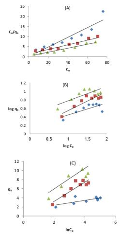
**Figure 8:** Langmuir (A), Freundlich (B), and Temkin (C) models of carmine dye adsorption onto activated carbon at 293k ( $\blacklozenge$ ), 298k ( $\blacksquare$ ), and 303K ( $\blacktriangle$ )
