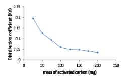
Figure 4: Effect of mass of activated carbon on E120 dye adsorption
