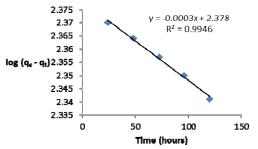
Figure 9: Pseudo-first- order kinetics for E120 dye adsorption onto activated carbons
