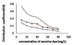
Figure 7: Effect of temperature on E120 dye adsorption onto activated carbon at 293 K (- $\bullet$ -), 298 K (- $\bullet$ -), and 303 K (- $\bullet$ -)
