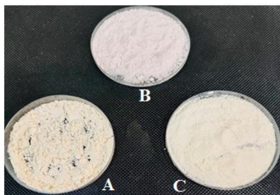
Figure 2: Photographic representation of the powdered formulations obtained after solidification of DC Na-ILs. BMIM-DC (a), Cho-DC (b), and BK-DC (c)
