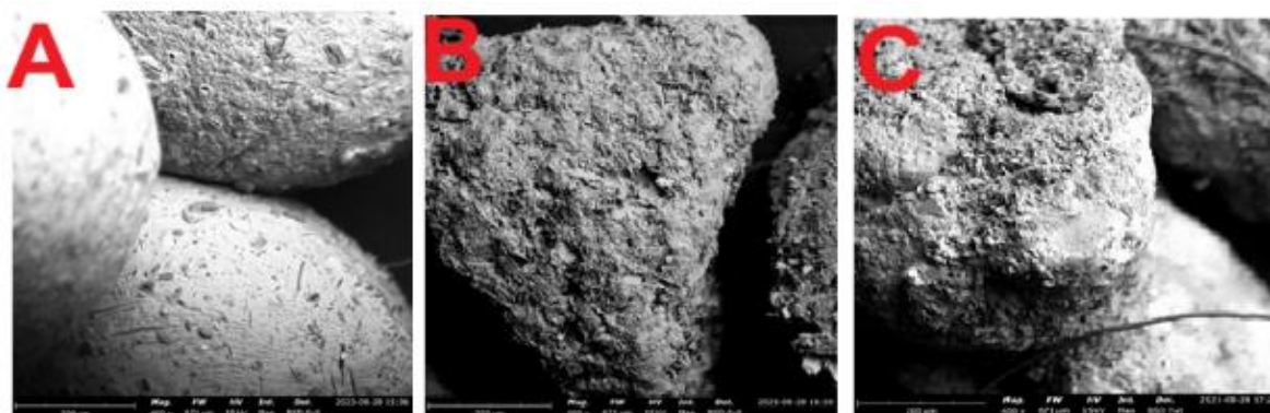
Figure 2: SEM of (A) Formulation M1 (microsphere containing alginate alone) (B) Formulation M5 (microsphere containing keratin + alginate in the core) (C) Formulation M9 (microsphere containing keratin in the gelling ion) Mag. 400 x
