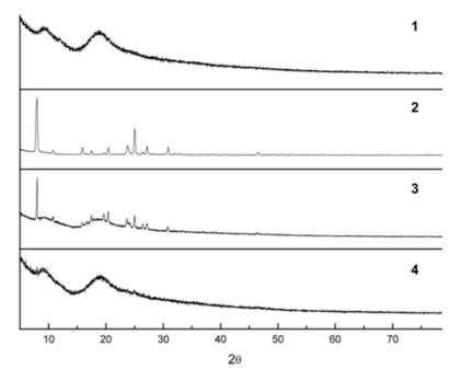
Figure 4: XRD patterns of HP- $\beta$ -CD (1), 4-hydroxylchalcone (2), their physical mixture (3) and complex (4)
