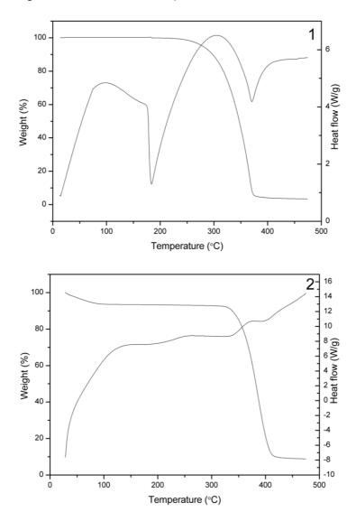
Figure 6: TG/DTA curves of 4'-hydroxylchalcone (1) and its complex (2)
