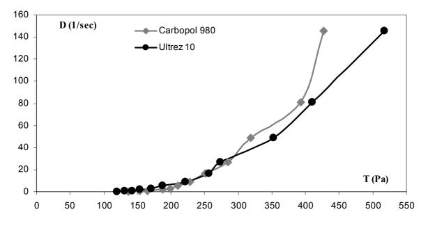
Figure 3: Flow curves of Carbopol gels after 100 days storage (n = 3)
