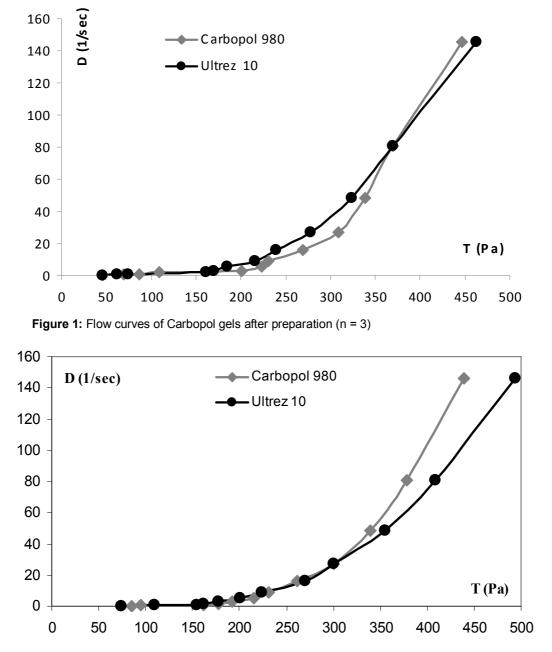
Figure 2: Flow curves of Carbopol gels after 50 days storage (n = 3)
